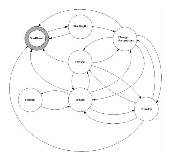
The device state can be retrieved with the functions *GetDeviceStateString* and *GetDeviceState*. Here is a brief description of the State of the FSM:
